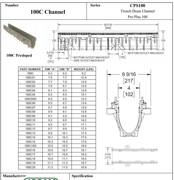
JOSAM 100C SERIES CHANNELS SHALL BE 39.4" (1000) LONG WITH 4" (102) INTERNALWIDTH AND RADIUSED BOTTOM. INTERCONNECTING CHANNEL SECTIONS SHALL BE MADE OF SMC/GRP (SHEET MOLDING COMPOUND/GLASS RE-INFORCED POLYESTER) MATERIAL AND AVAILABLE WITH AND WITHOUT SLOPE WITH INTEGRAL CHANNELSUPPORTS CAPABLE OF ACCEPTING RE-BAR. SUPPLIED BY TRENCH DRAIN SUPPLY.
